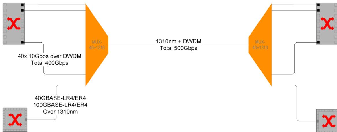
If this 1310nm band port is integrated into a 40 channel 100GHz DWDM passive multiplexer, then this set-up allows the transport of up to 40 services at 10Gbps plus 100Gbps over 1 fiber pair, in total 500Gbps, implemented into 1HU/19" rack space without consuming any electric power.
