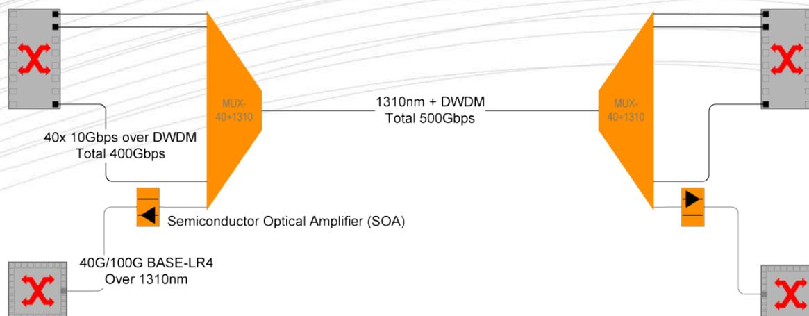
As with any amplified transmission here as well the signal quality and signal to noise ratio is of high importance. The SOAs therefore, have to be used as pre-amps (and not boosters) to amplify the incoming (Rx) signal on the receiving side of the link. Preferably and to extend reaches to the absolute maximum LR4 transceivers should be selected that exceed their specification in terms of signal quality. Doing so enables distances of up to 60km reach.
